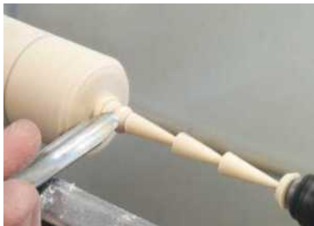
▲ Pic.5 The steps are cut in with the 10mm round skew. Present the point of the tool to the work with the handle low; as you lift the tool it will slice into the wood and give you great definition and a good finish
